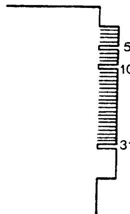
Figure 7 - 32- and 16-Channel Input Module Coding Cut-outs
